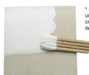
\* Mix the Batt Wash with water until a milky consistency and apply crosswise with a soft brush i.e. item no. 344121 in the picture.
