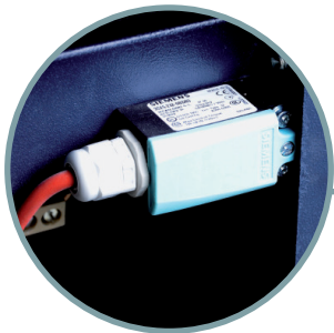
Forced safety switch connected to the lid.
